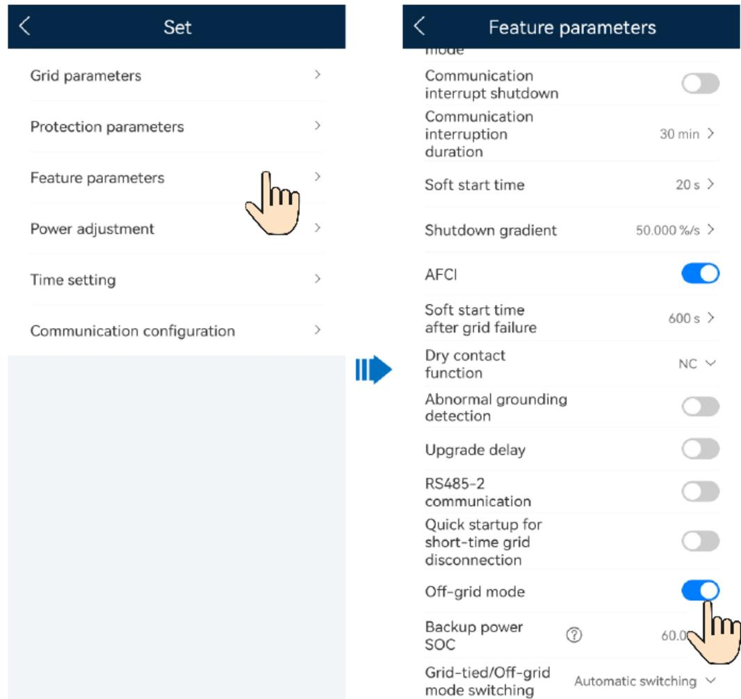
**Table 4-14** Parameter settings for grid-tied and off-grid operation
