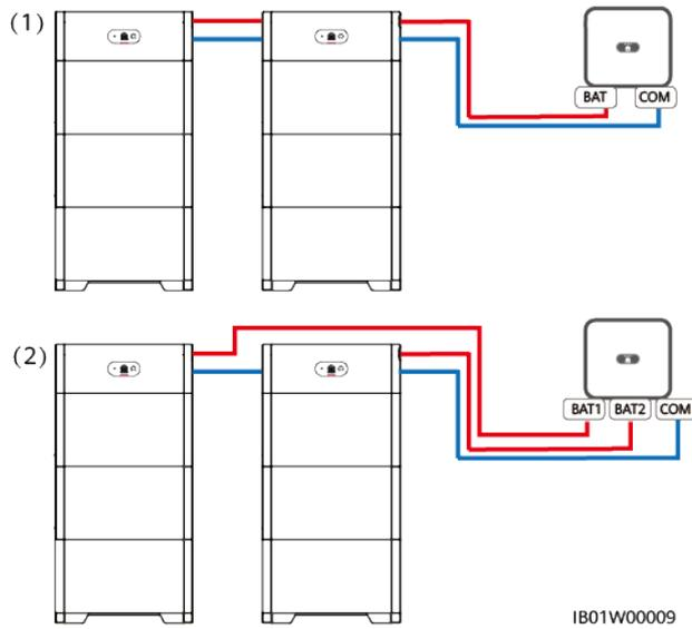
**Figure 6-19** Battery cascading cable connection (three batteries)
