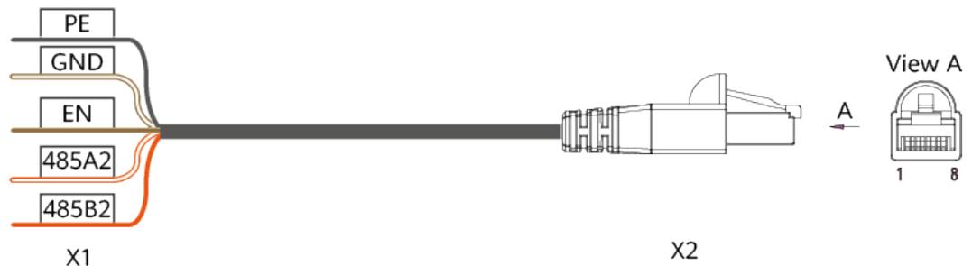
**Table 6-3** Signal cable connection (purchased from the supplier, type 2) between the battery and the inverter
