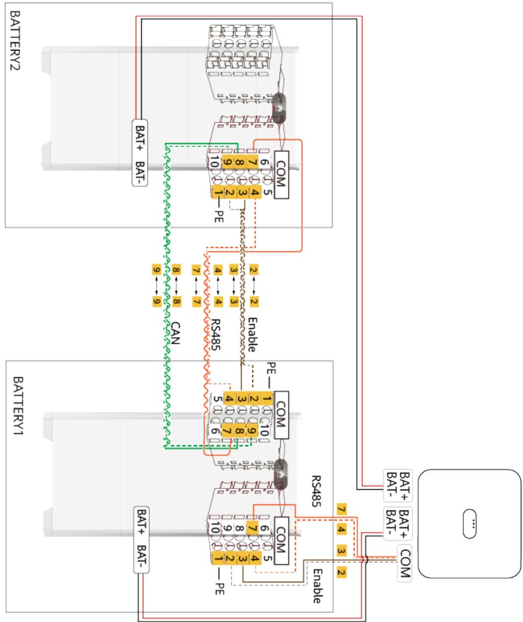
Figure C-4 Inverter connected to three batteries
