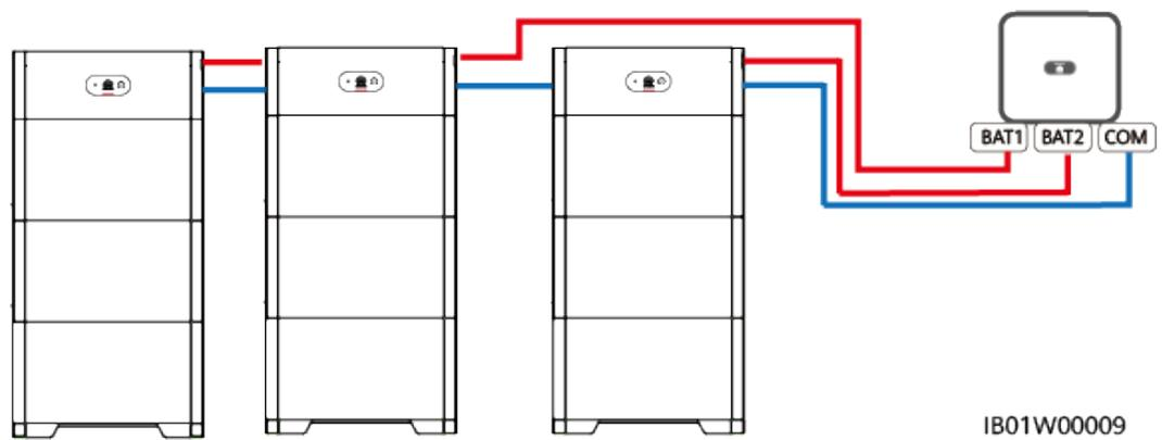
**Figure 6-20** Battery cascading cable connection (four batteries)
