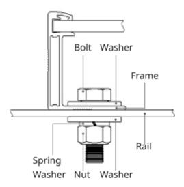
• Modules should be bolted at the following hole locations depending on the configuration and loads, which is shown in table 3.
