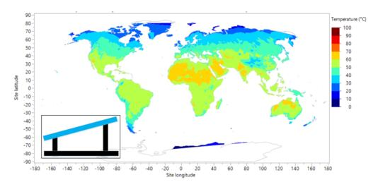
Figure A.1 – 98th-percentile temperature for an open-rack, or thermally unrestricted
