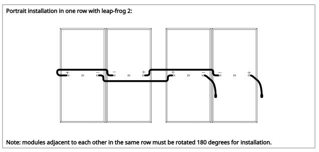
The maximum distance between two adjacent module frames should be within 50 mm (1.96 in) for the side with mounting clamps, and within 25 mm (0.98in) for the side without mounting clamps, in order to meet the system cable scheme.
