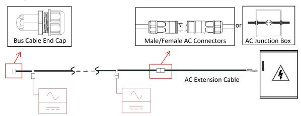
When an AC extension cable is required, users can either connect the AC bus cable and AC extension cable within a junction box or use a pair of male/female AC connectors provided by APsystems as optional accessories.
